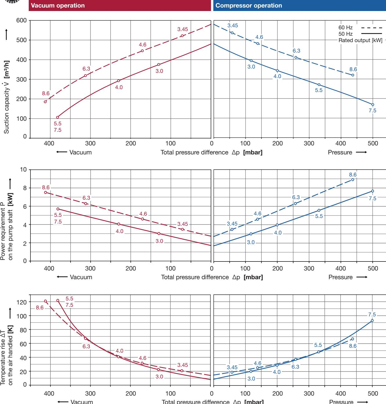
The performance curves are based on air at a temperature of 15 °C and an atmospheric pressure of 1013 mbar with a tolerance of  $\pm 10\%$ . The total pressure differences are valid for suction and ambient temperature up to 25 °C.
